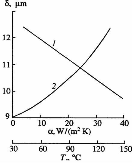
Fig. 2. Length of the diffusion zone as a function of (1) the heat-transfer coefficient and (2) the temperature of the ambient medium at  $t = 20s$ .
