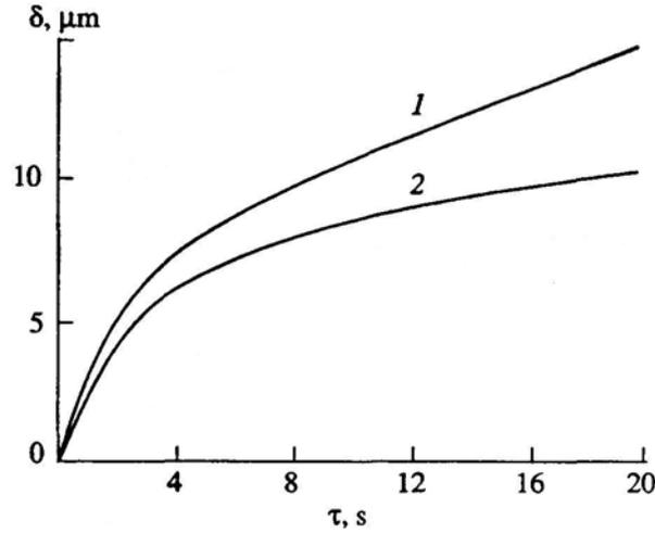
Fig. 1. Time dependence of the length of the diffusion zone: (1)  $D = \text{const}$ ; (2) with allowance made for  $D(T_g)$ .
